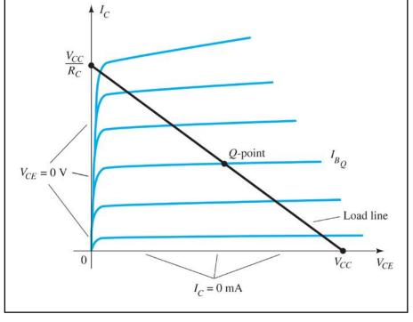
The Q-point is the operating point where the value of  $R_B$  sets the value of  $I_B$  that controls the values of  $V_{CE}$  and  $I_C$
