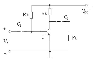
$$v_{ce} = -i_{c}(R_{C} /\!/ R_{L}) = -i_{c}R_{L}$$
