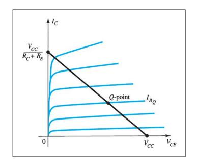
The endpoints can be determined from the load line.
