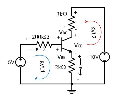
∴ Q1 is in active mode and the assumption is true we can also verify that the BC junction is reverse biassed which is required so that the BJT operates in active mode
