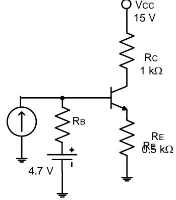
$$R_{ac} = R_{C} = 1 k\Omega$$
